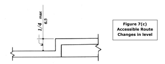
\*Cross section drawing showing a maximum 1/4 inch vertical change in level
