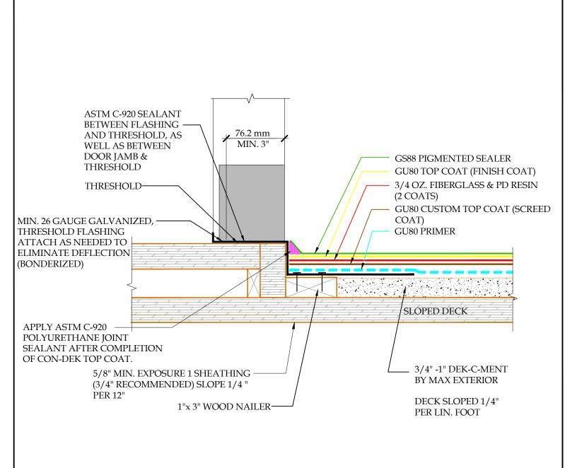
DETAIL-DEK-C-MENT BY MAX EXTERIOR-DOOR FLASHING
