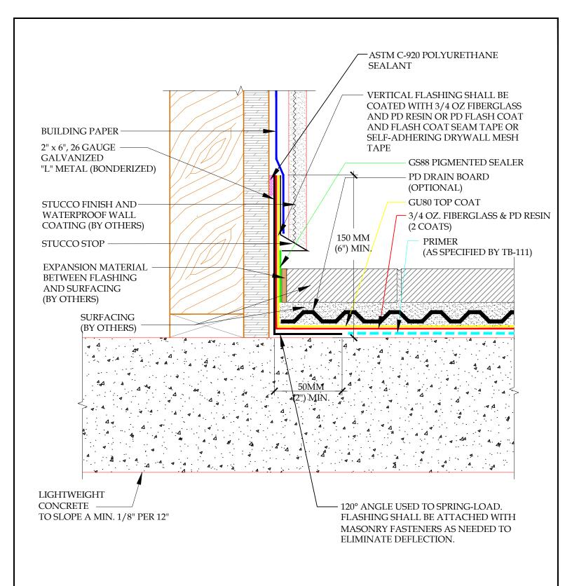
DETAIL-CON-DEK "U" SYSTEM - DECK TO WALL FLASHING-TILE OVERLAY SCALE: N.T.S.
