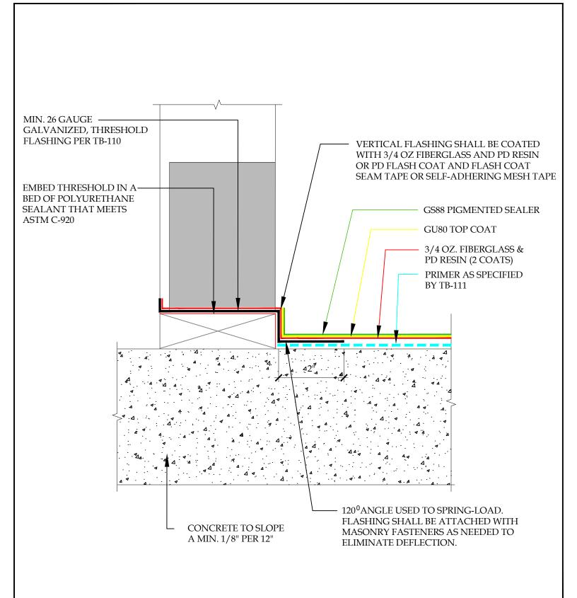
DETAIL-DOOR PAN FLASHING-ONE PIECE OVER CONCRETE SUBSTRATE - INCLEMENT WEATHER SCALE: N.T.S.
