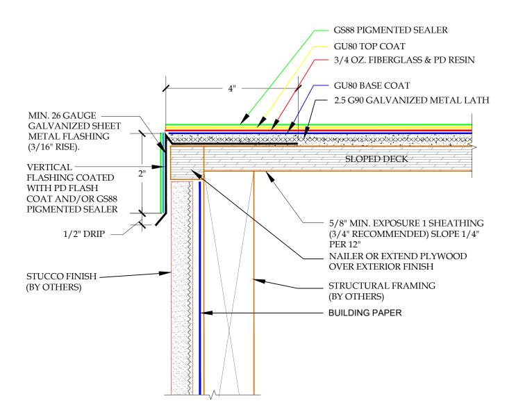
DETAIL-EDGE METAL FLASHING OVER STUCCO FASCIA-INCLEMENT WEATHER SCALE: N.T.S.
