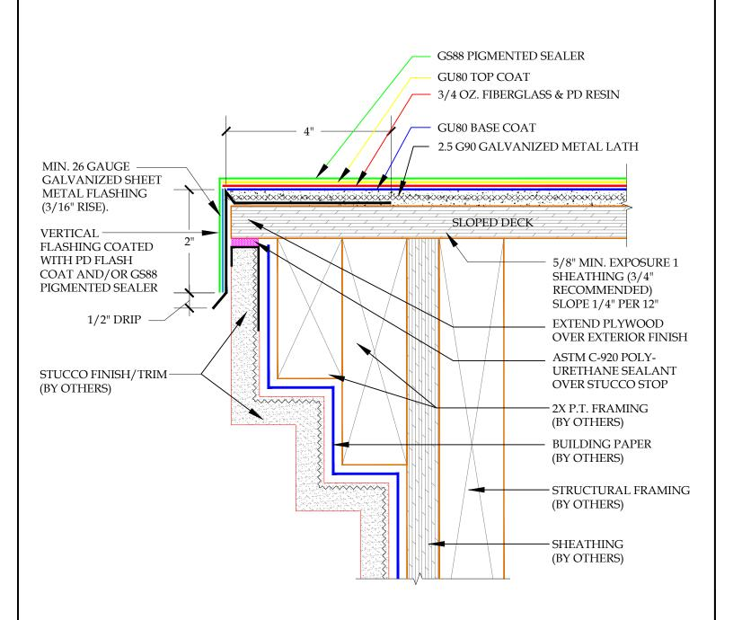
DETAIL-EDGE METAL FLASHING OVER STUCCO TRIM BAND - INCLEMENT WEATHER SCALE: N.T.S.
