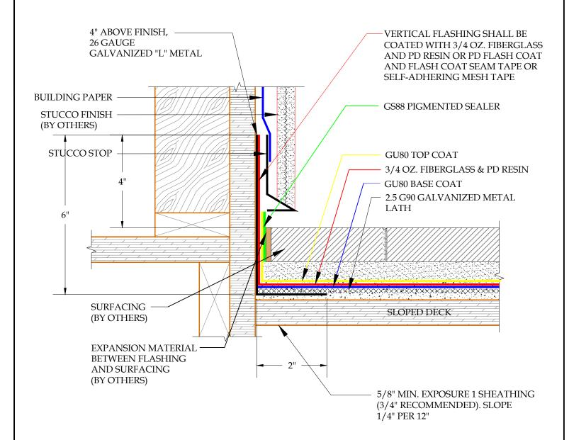
DETAIL-PLI-DEK "U" SYSTEM-DECK TO WALL FLASHING DETAIL-SURFACING OR CONCRETE OVERLAY - INCLEMENT WEATHER SCALE: N.T.S
