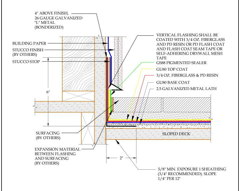
DETAIL-PLI-DEK "U" SYSTEM- DECK TO WALL FLASHING DETAIL-SURFACE OR CONCRETE OVERLAY SCALE: N.T.S
