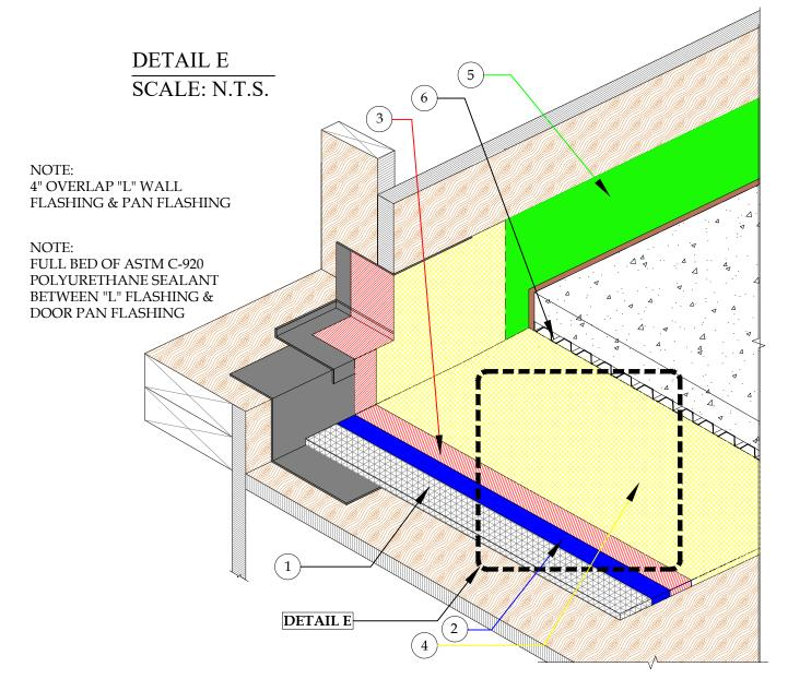
DETAIL-PLI-DEK "U" SYSTEM - MASONRY OR CONCRETE OVERLAY - INCLEMENT WEATHER SCALE: N.T.S.
