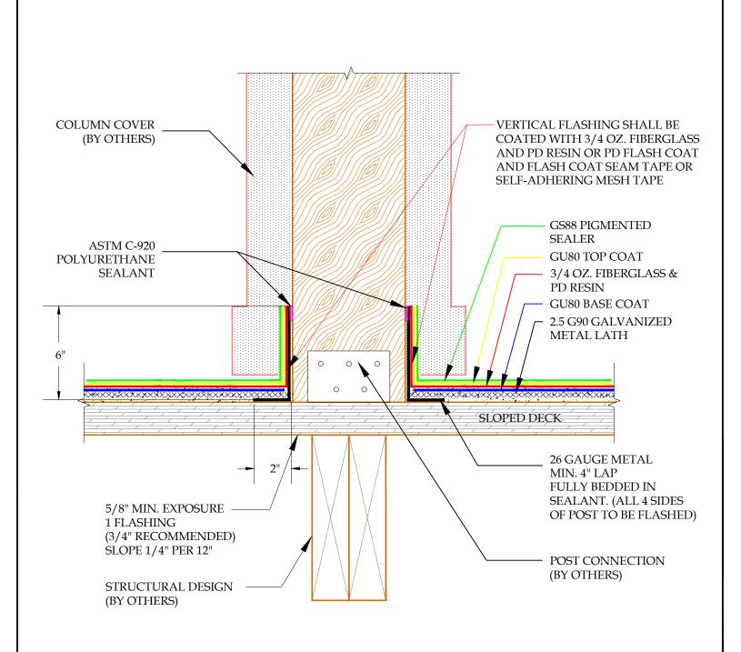
DETAIL-WOOD POST FLASHING WITH COLUMN COVER - INCLEMENT WEATHER SCALE: N.T.S.
