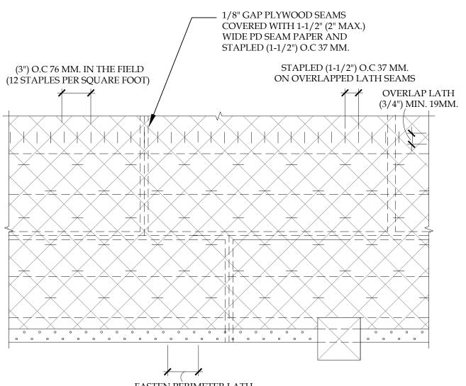
FASTEN PÈRIMETER LATH METAL (1-1/2") O.C 50MM-2 ROWS STAGGERED
