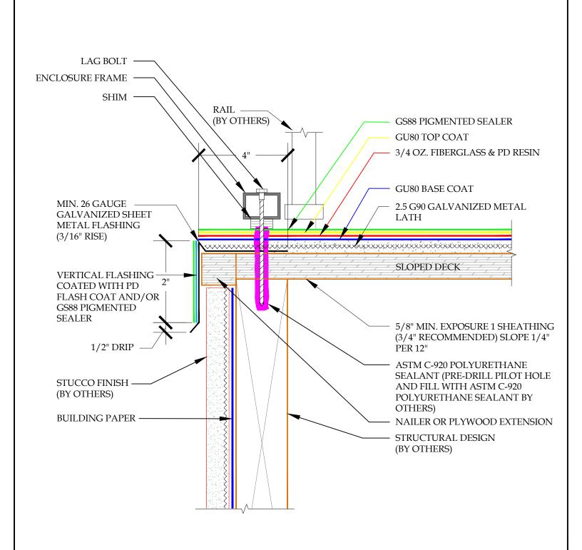
DETAIL-PERIMETER DECK FLASHING DETAIL-ENCLOSURE ATTACHMENT-INCLEMENT WEATHER SCALE: N.T.S.
