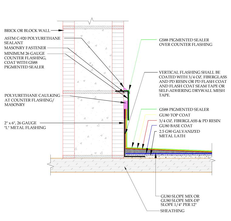
DETAIL-BLOCK/BRICK TO DECK SLOPE-INCLEMENT WEATHER SCALE: N.T.S.
