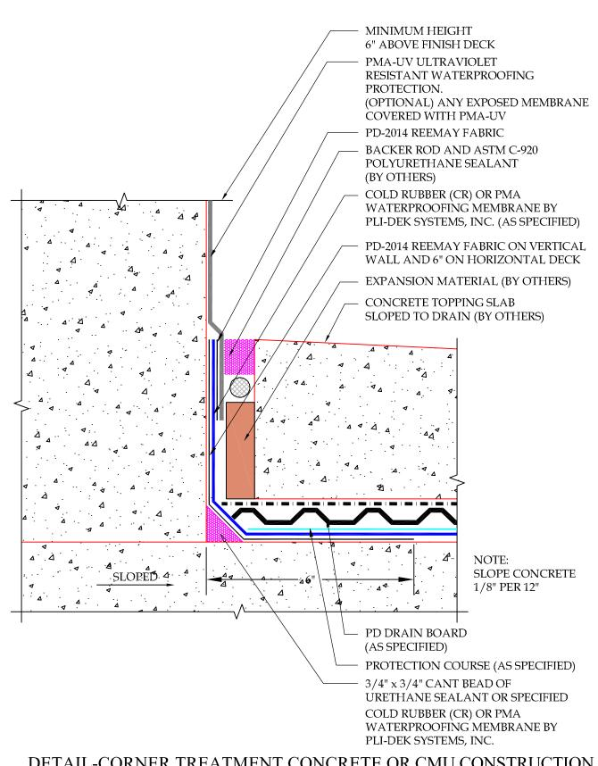
DETAIL-CORNER TREATMENT CONCRETE OR CMU CONSTRUCTION SCALE: N.T.S.
