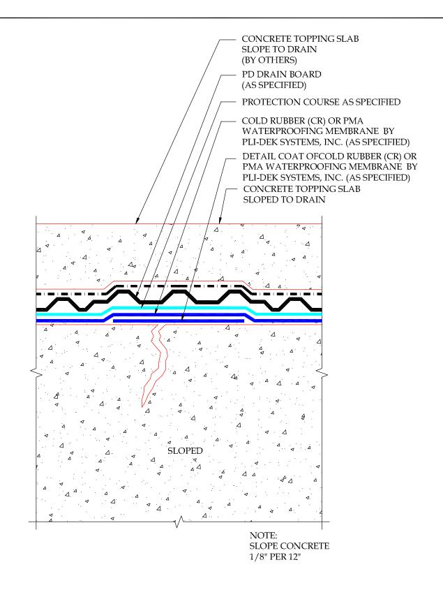
DETAIL-TREATMENT OF CRACKS LESS THAN 1/8" SCALE: N.T.S.
